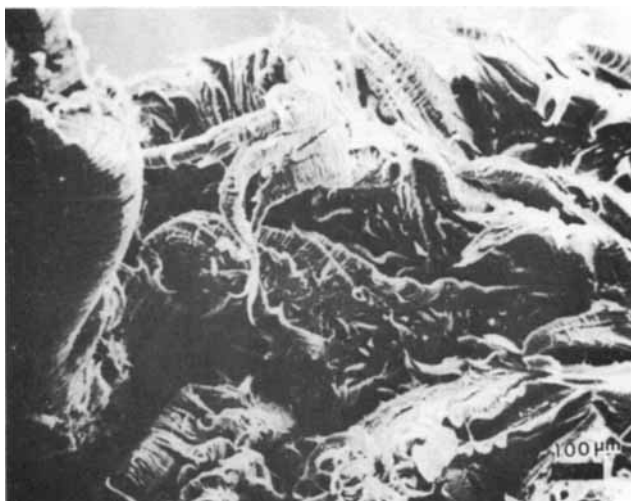
Fig. 2. Fracture surface of LDPE sample drawn in methanol at 60°C.
