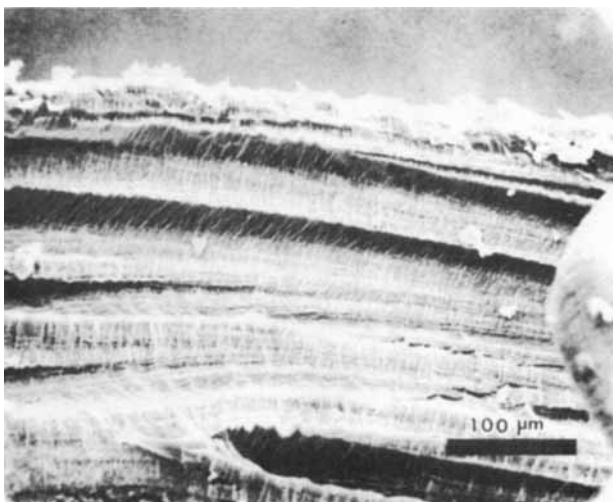
Fig. 3. Fracture surface of LDPE sample drawn in water at 60°C.
